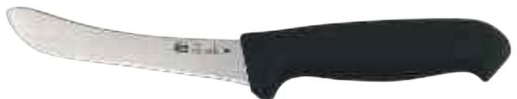
Blade: Blade made of Swedish cold-rolled stainless steel. Hardened by deep refrigeration at -80 degrees for maximum hardness. Hardness: 58 RC.
