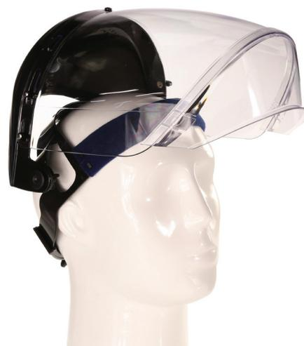
The REON™ face shield provides the wear with 'Class A' face protection. High energy impact resistance to EN 166 'Level A' means that the face shield protects against impacts up to 190m/s (425mph). REON is also top of the class for comfort and vision clarity.
