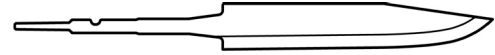
Morakniv Knife blade No. 3 | Carbon Full rat tail tang with blade of carbon steel.
