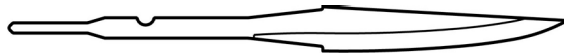
Morakniv Knife blade No. 106 | Laminated Full rat tail tang with blade of laminated carbon steel.
