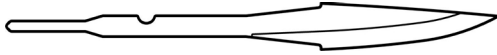
Morakniv Knife blade No. 120 Full rat tail tang with blade of laminated carbon steel.
